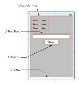
**FIGURE 6-2:** Annotated UIKit elements in Scrambler
