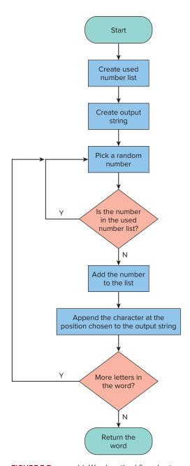
FIGURE 5-7: scrambleWord method flowchart
