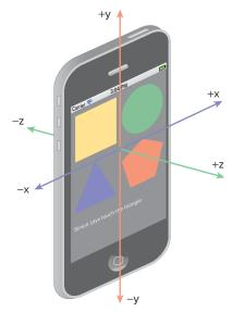
FIGURE 7-5: Accelerometer coordinate system
