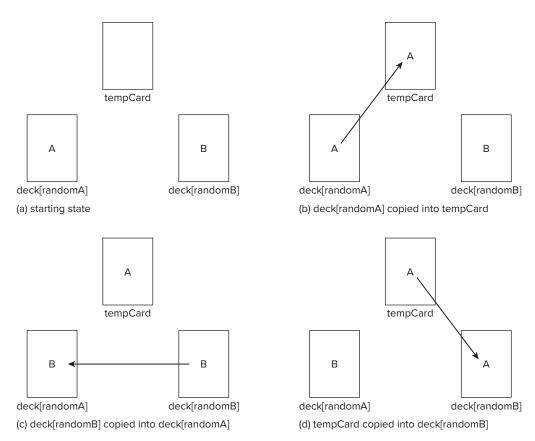
FIGURE 3-8: Swapping values with a temp variable
