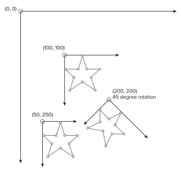
FIGURE 6-8: Translation and rotation of the coordinate system
